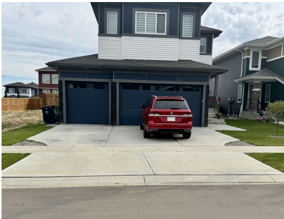
Not permitted, curve on both sides must be 6' from PL
